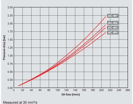
Measured at 30 mm<sup>2</sup>/s Tolerance: ±5%
