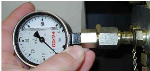
Attach the pressure gauge to test point 1.
