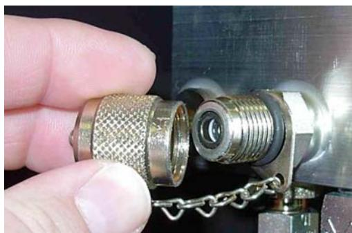
Close both test points 1 + 2 using the connected dust cap.
