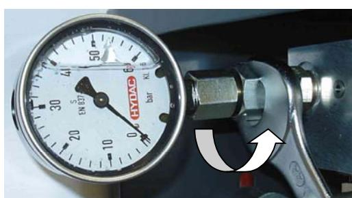
Remove the pressure gauge from test point 1 and connect it to test point 2 **[C]**.
