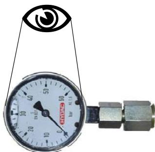
Set the pressure at maximum viscosity of the hydraulic medium to ca. 25 bars.
