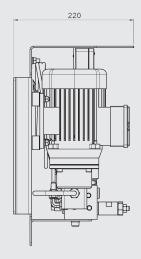
CMP with gear pump, fluid sensors MCS1310 and HLB1400 and data logger / network interface CSI-C-11
