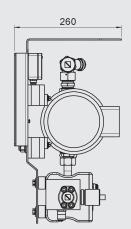
CMP without motor pump assembly, fluid sensors CS1220 and HLB1400 and data logger / network interface CSI-C-11
