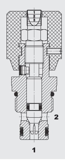
The needle valve is a direct-acting valve which controls the flow rate by adjusting the cross section. The flow rate is dependent on the pressure differential and the viscosity.
