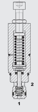
The pressure sequence valve is a direct-acting, spring-loaded poppet valve with built-in check valve. In the normal position, the path from port 1 to port 2 is blocked.
