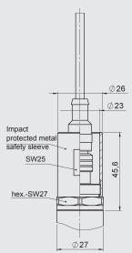
The impact protected metal safety sleeve is included. A straight female connector is required for electrical connection; e.g. female connector M12x1, 4 pole, straight, with 3m shielded cable: ZBE 06S-03, Part No. 6098243
