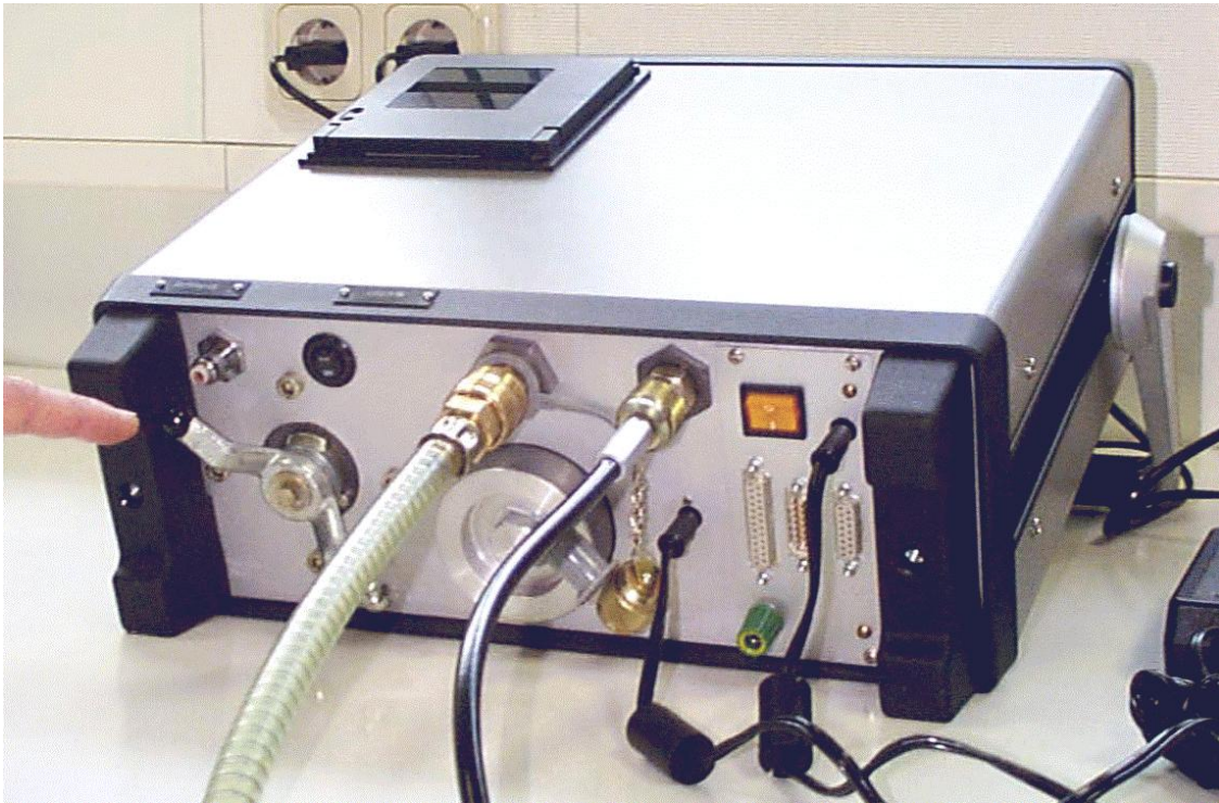
Figure 7 : Setup for measurements with high pressure inlet
