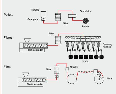
Application schematic for production of pellets, fibres and films
