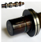
Valve piston with deposits
