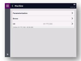
If the controller is disconnected from the CANbus, the HMG switches back to the machine menu and the status will be displayed as "Offline".
