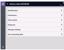
After having selected "Parameters", the individual parameters can be opened or modified for the output data by tapping the corresponding button.
