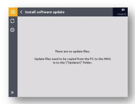
Update files for the device always have to be transferred manually from the PC to the HMG 4000 and into the folder "HMG / Updates". Multiple update files can be saved to the device at the same time.
