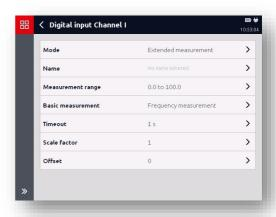
The measured value is calculated by multiplying a basic measured value with a scaling factor and then adding an eventual offset value to this.
