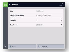
After tapping "Continue", the connected device is configured with the changed settings.
