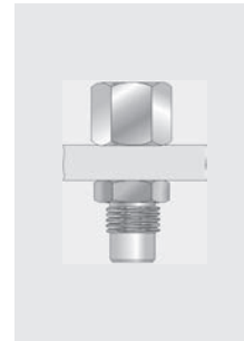
Pressure gauge connection for bulkhead pipe fitting
