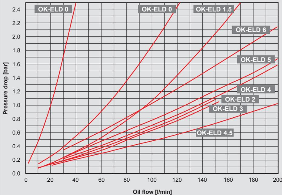
measured at  $30\text{ mm}^2/\text{s}$
