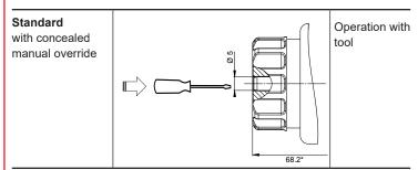
\* Dimensions up to valve casing
