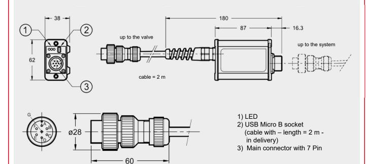
In the casing of electronics, a 7-pole port for connecting with external devices is integrated.
