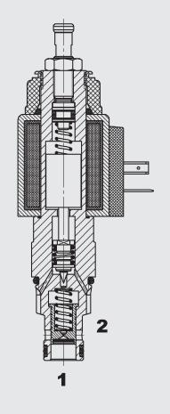
The PDB10PZ is a pilot-operated, spool type proportional pressure relief valve. If pressure at port 1 exceeds the setting defined by the electrical signal, the pilot poppet opens and oil flows from behind the main spool to tank port 2. The resulting pressure differential causes the main spool to lift against the return spring and allows flow from port 1 to port 2. As a function of the electrical signal, the relief pressure at port 1 can be changed steplessly.
