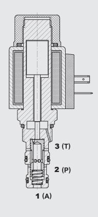
**3-Way Proportional Pressure Reducing Valve** Spool Type, Direct Acting UNF Cartridge – 350 bar PDR08-02
