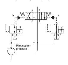
The valve has been specially developed for pilot applications. In these applications, the main requirement is precise conversion of the input signals to a stable control pressure. At the same time, the leakage during the control procedure must remain low, to ensure that the hydraulic accumulator can preserve the emergency supply of the pilot control circuit for as long as possible in the event of an error.
