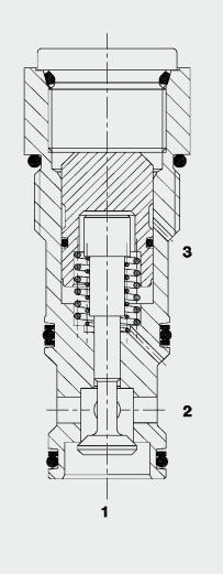
The pilot-to-open check valve RP16A is a direct-acting, spring-loaded poppet valve.
