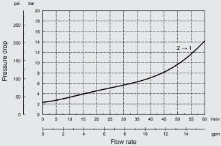
Throttle curve: ∆p-Q from port 1→2 maximum control
