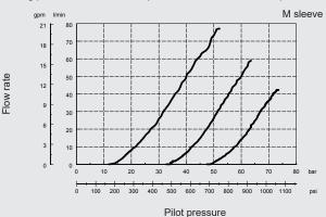
**Throttle curve:**  $\Delta p$ -Q from 2 to 1
