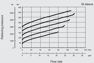
**Pilot curve:** volume flow from 1 to 2 via pilot pressure at 3 The pilot control function shows the lowering speed on the pilot pressure. Setting pressure: 200 bar; Load pressure: 25, 50, 85 % of set pressure
