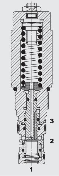
The counter balance valve is a direct acting poppet valve. It has to control the lowering speed according to the supply flow rate. It also prevents the consumer from hurrying on ahead when there are pulling loads and allows a jerk-free movement of the same. It also carries out the function of a hose-break valve. For details about the functionality, see page 3.
