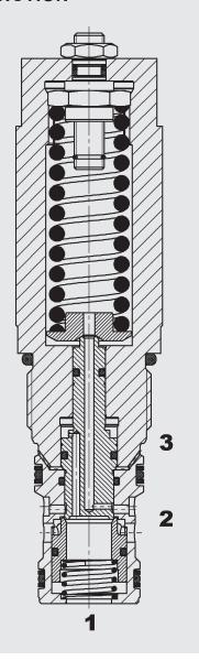
The counter balance valve is a direct acting poppet valve. It has to control the lowering speed according to the supply flow rate. It also prevents the consumer from hurrying on ahead when there are pulling loads and allows a jerk-free movement of the same. It also carries out the function of a hose-break valve. For details about the functionality, see page 3.
