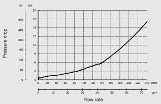
Throttle curve: ∆p-Q from port 1→2 maximum pilot control
