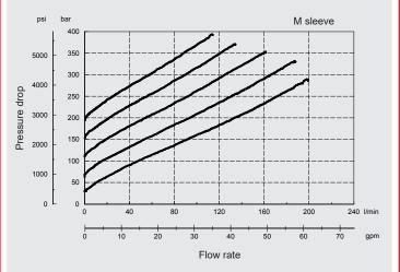
Pilot curve: (flow from 1 to 2 via pilot pressure to 3) The pilot function shows the lowering speed on the pilot control pressure. Setting pressure: 200 bar; Load pressure: 25, 50, 85% of set pressure
