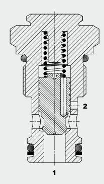
**Check Valve Poppet Type Metric Cartridge – 350 bar** RVM10120-51
