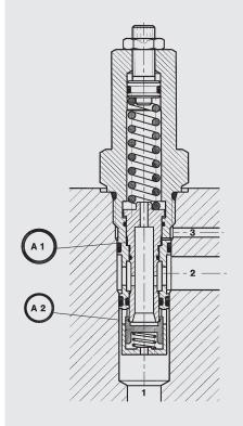
Counterbalance valves are direct-acting poppet valves with integrated check valve which enable smooth action of loads if there are retracting and extending loads. In loadholding applications, it can be used as a hosebreak valve.
