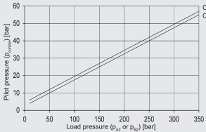
Cracking pressure = 4 bar Cracking pressure = 2 bar
