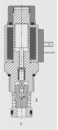
When de-energized, there is free flow through the valve from port 2 to 1. Flow in the opposite direction is not permitted. When energized, the valve is closed from port 2 to port 1. In the reverse direction there is free flow
