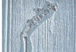
Fig. 6: Embedded machining chip
