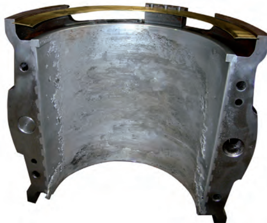
Fig. 4: Melted white material caused by solid particle contamination and increases in temperature
