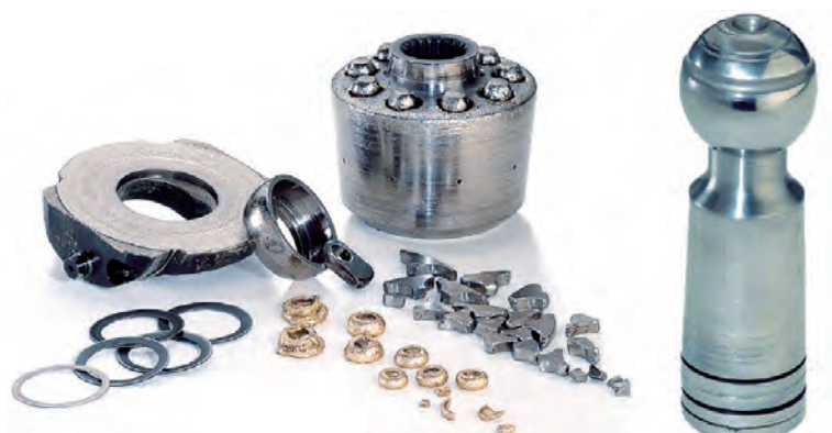
Fig. 5: Damage to the components of a variable displacement pump
