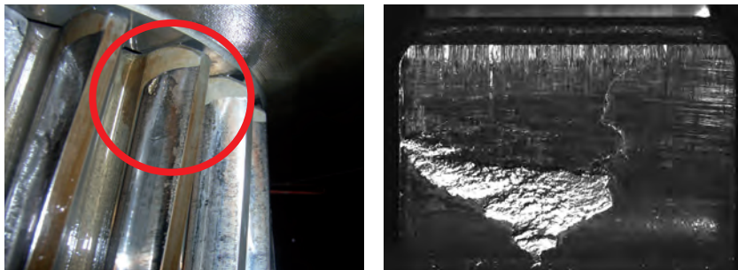
Figs. 2+3: Damage to a gear rim
