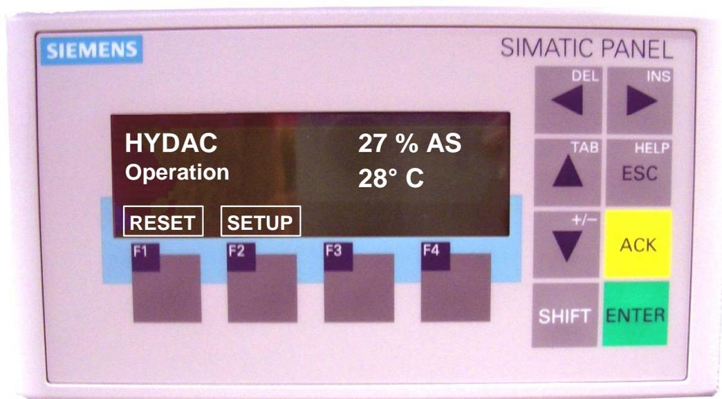
In the event of error messages, it is possible to jump back to the text display by pressing the TAB key.
