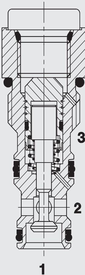
The pilot-to-open check valve is a direct-acting, spring-loaded poppet valve. The valve allows flow from port 2 to 1. In the opposite direction, the poppet is pressed onto the seat and blocks flow. If a sufficiently high control pressure is applied at port 3, the poppet is lifted from the valve seat and oil flows from 1 to 2. The necessary pilot pressure at port 3 is dependent on the pressures across port 1 and 2.
