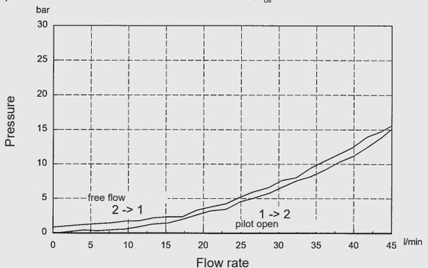
phi=4:1 measured at  $v = 34 \text{ mm}^2/\text{s}, T_{oil} = 46 \text{ }^\circ\text{C}$
