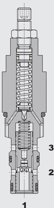
The DR10P is a pilot-operated, spring-loaded, spool type pressure reducing valve.
