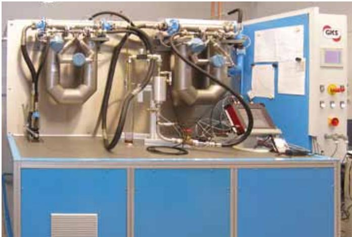
Test rig for characterisation of air separators
