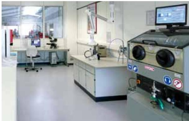
HYDAC conducts component cleanliness analyses in the FluidCareCenter in accordance with the various current standards (ISO 16232 and VDA Volume 19), factory standards as well as customer specifications.
