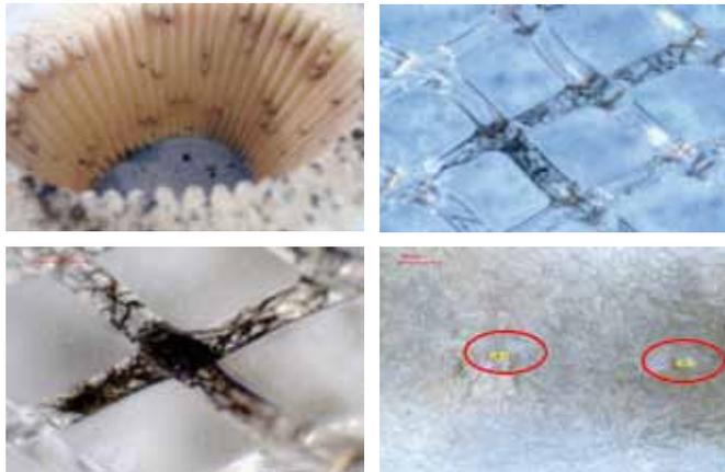
Damage due to electrostatic discharge on the **filter element**
