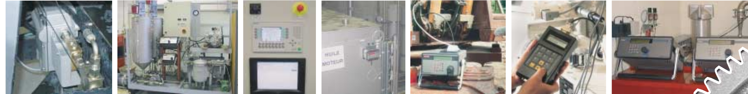
Contamination Sensor On board Contamination test bench Contamination control Software CoCoS Temperature monitoring Measurement of the contamination using FCU Multi-function portable data recorder HMG Cleanliness monitoring during filling
