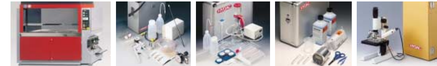
CTU 2000 series Contamination Test Unit FES Fluid Extraction Set FAS Fluid Analysis Set WTK 200 Water Test Kit MM S5 Measuring microscope
