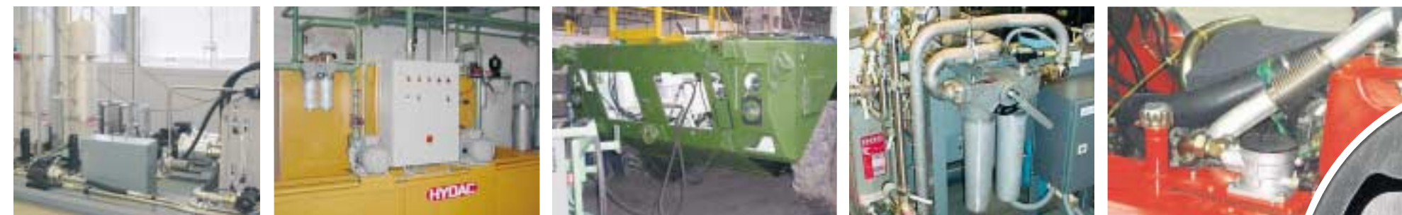
Test rig Filling unit Flushing on military tank system Change-over low pressure filter FLND Return line & suction boost filter RKM
