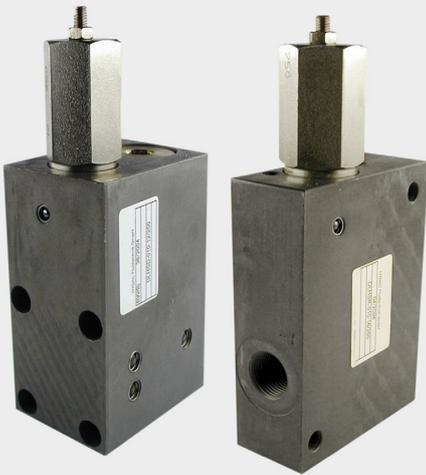
The accumulator charging valve DLHSD / R is a pilot-operated, spring-loaded spool valve mounted in a manifold or inline housing. Its function is to control the charging of the accumulator within a pre-set switching range. A pilot stage with defined hysteresis, a main piston and a check valve are integrated into the circuit.
