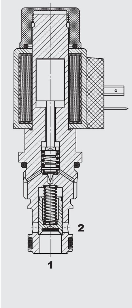
The PDB12P is a pilot-operated, spool type proportional pressure relief valve. If pressure at port 1 exceeds the setting defined by the electrical signal, the pilot poppet opens and oil flows from behind the main spool to tank port 2. The resulting pressure differential causes the main spool to lift against the return spring and allows flow from port 1 to port 2. As a function of the electrical signal, the relief pressure at port 1 can be changed steplessly.
