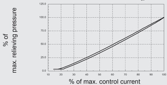
Measured at  $v = 34 \text{ mm}^2/\text{s}$ ,  $T_{\text{oil}} = 46^\circ \text{C}$
