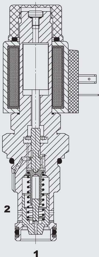
The PWK12120WP is a normally closed, spool type, pilot-operated proportional flow control valve. Together with a pressure compensator, which maintains a constant differential between the inlet pressure (port 1) and the outlet pressure (port 2), it can be used as a proportional flow regulator.
