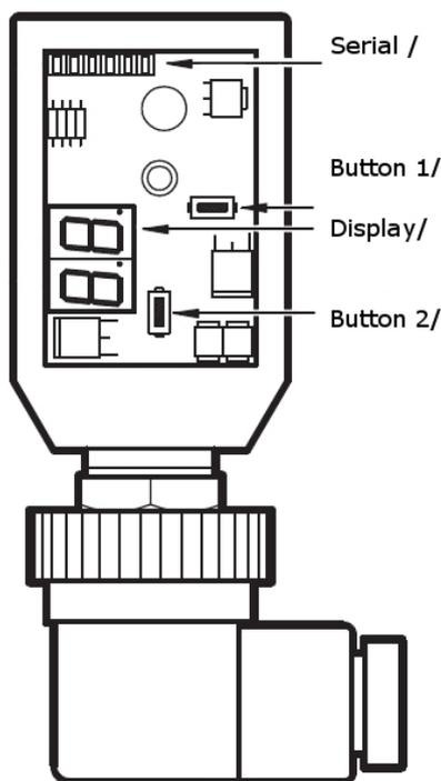
The picture shows the open plug amplifier. Only in this mode it is possible to operate the buttons. The LED display is also visible with closed cover.
