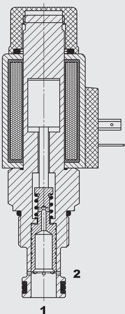
The PWK10120V is a normally open, direct-acting, spool type, 2-way proportional flow control valve. Its function is to smoothly control the flow from port 1 to port 2. The electrical signal reduces or increases an orifice cross-section. Together with a pressure compensator it is used as a full flow regulator, for example to lift and lower variable loads at the same velocity.
