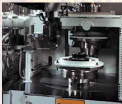
Electron-beam welding of diaphragm accumulators
