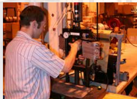
Precharging of a Diaphragm Accumulator
