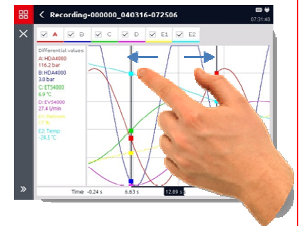
Fig.: Using the magnifying gesture with two fingers, the operation is carried out - Zooming in this case.
