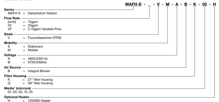
\* = K filter housing will use the GeoSeal elements Q filter housing will use the 39QCLQF Filter Systems elements
