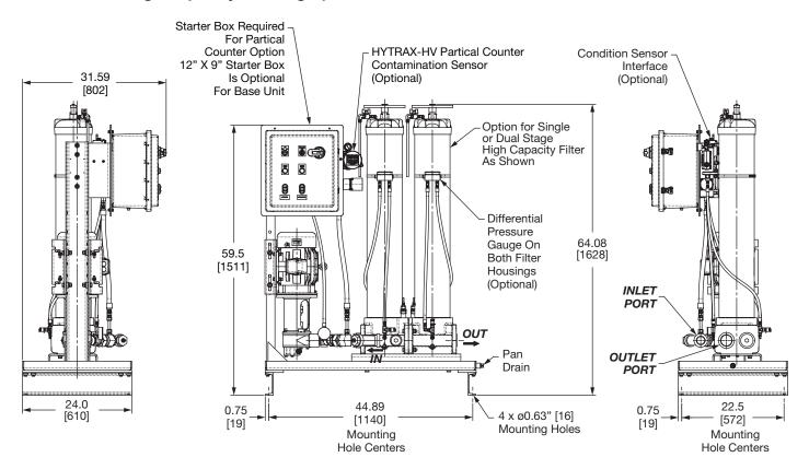
Dimensions are for general information only, all critical dimensions should be verified by requesting a certified print. Dimensions shown are in inches [millimeters].
