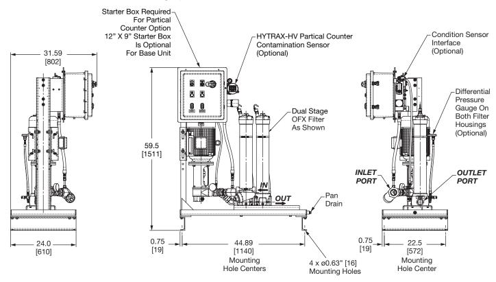
Dimensions Dual OFX5 Series with the H3 - high capacity housing option
