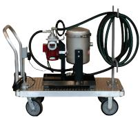
The filter unit is equipped with a CS1000 contamination sensor and CSI-C-11 condition sensor interface and needs to be ordered with new element. Flow rate is 5 GPM and is ideal for reservoir volumes up to 2000 liters. Power supply 120 VAC/1ph/60Hz. Power cord (approx. 30 feet). Comes on a mobile cart with casters. Suction and return hoses included, size ¾ inch, with female JIC ends, length of hoses is 15 feet.
