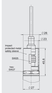
The impact protected metal safety sleeve is included. A straight female connector is required for electrical connection. e.g. female connector M12x1, 4 pole, straight, with 3m shielded cable: ZBE 06S-03, Part. No. 6098243
