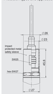
The impact protected metal safety sleeve is included. A straight female connector is required for electrical connection. e.g. female connector M12x1, 4 pole, straight, with 3m shielded cable: ZBE 06S-03, Part. No. 6098243
