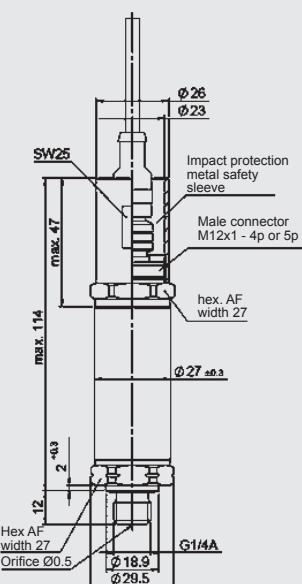
The impact protection metal safety sleeve is included. A straight mating connector is required for electrical connection. E.g. mating connector M12x1, 4 pole, with 3 m shielded cable: ZBE 06S-03, part no. 6098243
