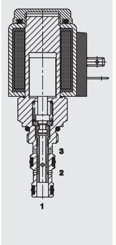
When the solenoid coil is de-energized, the valve allows flow from port 1 to 2 or from port 2 to 1, while blocking flow at port 3. When energized, the valve allows flow from port 3 to 1 or from port 1 to 3, while blocking flow at port 2. **3/2 Solenoid Directional Valve UNF Spool Type, Direct-Acting SAE-07 Cartridge – 350 bar** WK07L-01
