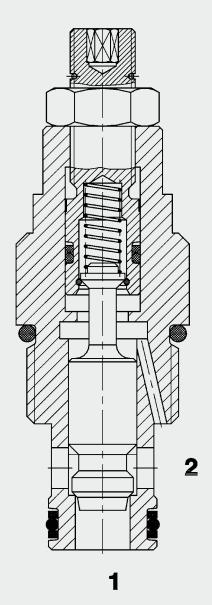
The SDR10A controls flow from port 2 to port 1 and is non pressure compensated. That means the flow rate depends on the pressure differential and viscosity. There is free flow from port 1 to port 2.
