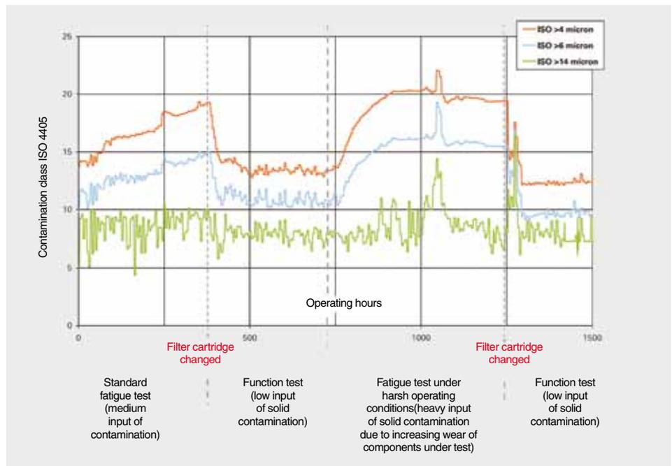
**Fig. 7:** Levels of contamination according to ISO classification and the change in levels
