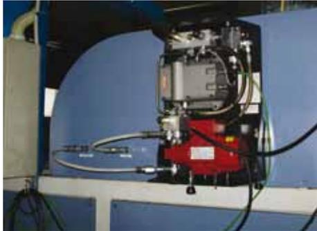
**Fig. 3:** HYDAC Module CSM 2000, installed next to the tank on test rig in the R&D department. To the left, connections (IN/OUT) to the tank.
