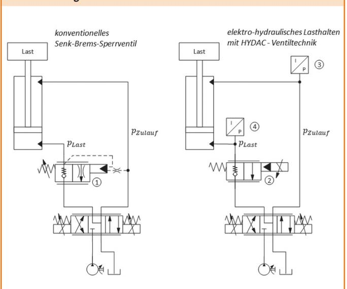
02 Inlet pressure in relation to load pressure
